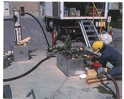
Fuel filtration is one method that can be used to treat stored fuel by removing particulate matter which has accumulated over time.
