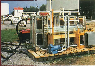
Development and operation of totally enclosed treatment system for benzene in tank bottoms.
