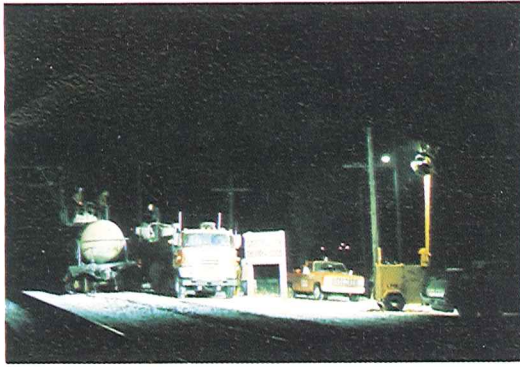
This 8,000 gallon tank car of 90% Hydrogen Peroxide derailed inside a town and forced the evacuation of 2,000 people. O. H. Materials successfully patched the leaking car and transferred the uncontaminated load.
