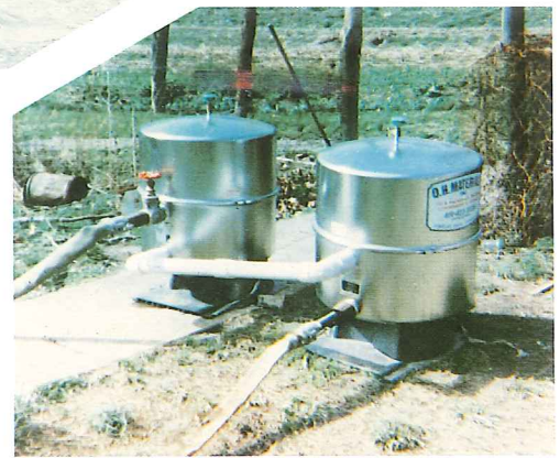
Mobile carbon filtration systems are rapidly deployed and installed at spill sites for removal of organic pollutants.
