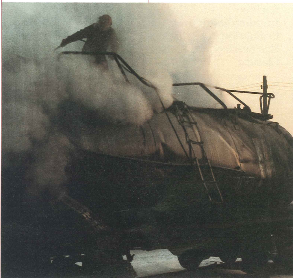
Tank car patching prior to product transfer
