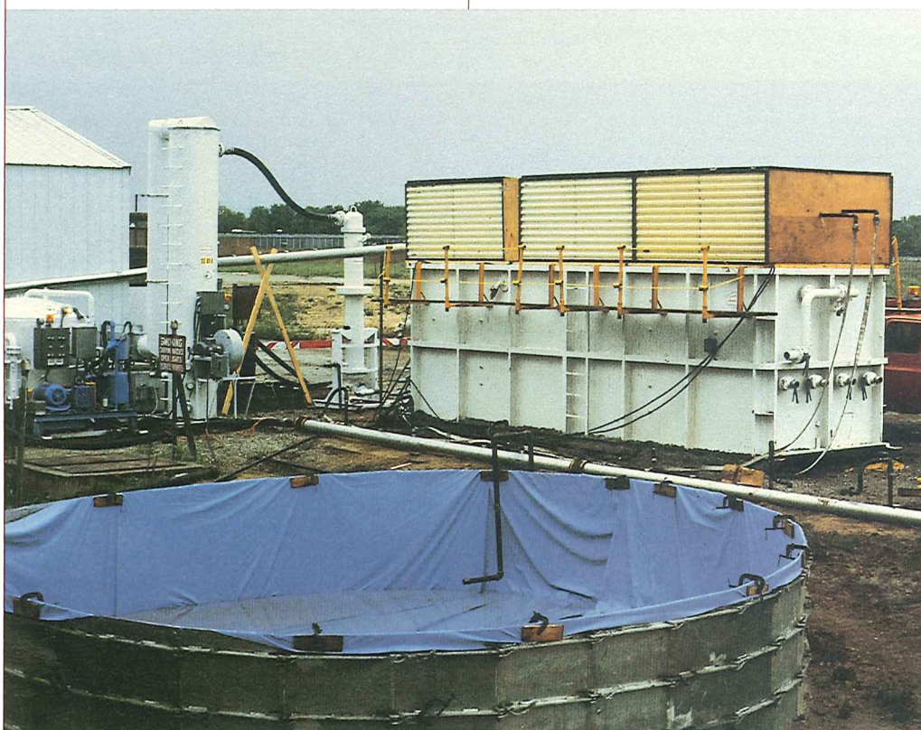
Mobile treatment system — clarifier, retention pool and air stripper
