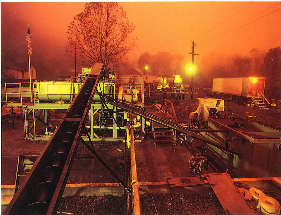
Extractions of contaminants from soil using custom-designed on-site treatment or destruction technology.
