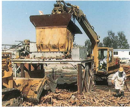
Mobile shredders can be used as volume reduction and cost-saving tools.
