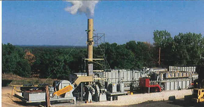
PCB destruction using OHM's TSCA-permitted incinerator to treat 3,000 tons of soil at the Twin Cities Army Ammunition Plant, Minnesota.
