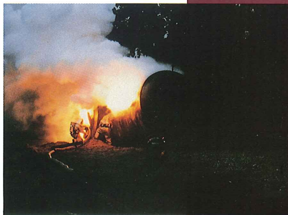
Controlled burn and monitoring program for 23,000 gallons of white phosphorous in a derailed tank car.
