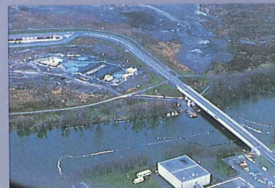
(Above series) Dredging of coal-tar-contaminated river sediments for dewatering, water treatment, and disposal. Sediments were removed from the Rideau River in downtown Ottawa, Ontario, and treated to meet Ministry of Environment provincial discharge criteria.
