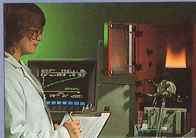
Trace heavy metal environmental analysis using state-of-the-art methods including Zeeman/Graphite Furnace Atomic Absorption.
