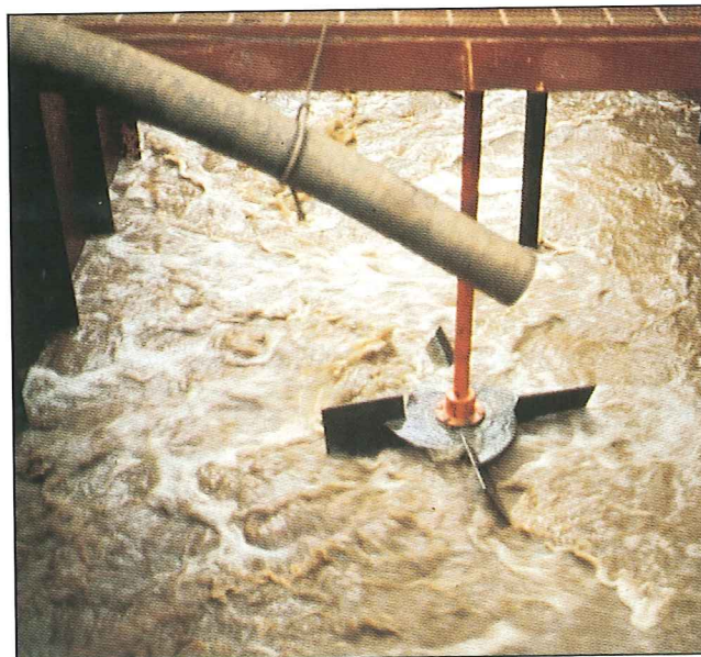
FIGURE 5. This soil-washing unit serves to reduce the volume of soil needing further biotreatment
