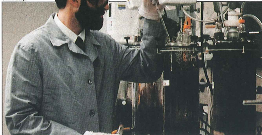
FIGURE 1. Laboratory studies in bioreactors usually precede actual soil treatment
