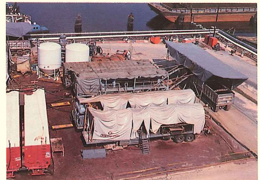
Recessed chamber filter presses reduced river sediment volumes by 54 percent
